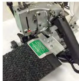
Bond Model PBB-1X applying transition molding on an entrance mat.
