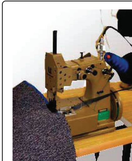
Model HDS & HDSB Heavy Duty Serger (STK#21990X, STK#21990BX) Heavy duty wrap around table serger with binder. The most heavy duty serger on the market, bar-none. Uses one spool of tex 210 bonded nylon and the serging yarn of your choice. Bind and serge in one pass operation.
