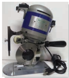
Bond Model HDC-5 (STK#21910) 5" Heavy Duty Rotary Straight Cutter Self Sharpening 110v AC
